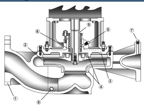
**1.Casing** - Flanged suction and discharge on common centerline. Integral one-piece unit suitable for in-line or pedestal mounting. Designed for working pressures up to 350 PSI with 1/4" corrosion
